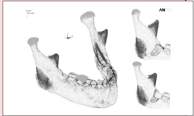
Figure 6: Boundary conditions for the three cases with ipsilateral loading of the first molar. In case 1 (large mandible on the left), the third molar is still in place. In case 2 (partial mandible, top right), only the right third molar has been removed, without removal of the cortical bone. In case 3 (partial mandible, bottom right), the right third molar has been removed, along with the necessary cortical bone, mainly around the crown of the tooth and at the lateral cortical wall in the area of the external oblique ridge.
