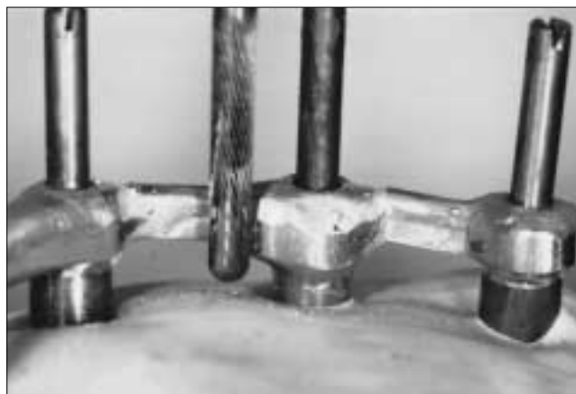
Figure 2: Final milling of the cast bar.
