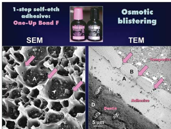
Figure 9: Scanning and transmission electron micrographs of water blisters that formed along the self-cured composite interface with single-step adhesives; these blisters resulted in very weak bonds and premature failure of the adhesive. Adapted from Tay and others. 54
